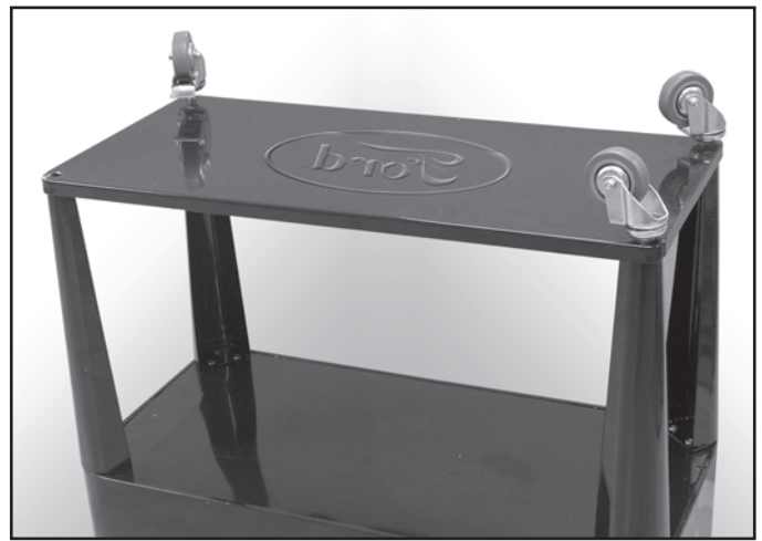
Step 4: Screw wheels into legs. Locking casters on same side. Now go back and tighten screws holding legs. Once done stand cooler upright.
